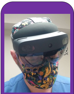
Figure 1. Closeup of the Augmented Reality device (HoloLens 2, Microsoft); Shows integrated cameras and the display.
